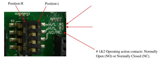
Modbus return the status of the three micro-switches and dry contacts of a virtual or real analog board based on threshold settings. Hystereses of contacts: CO2: 100ppm, VOC: 10% of the formaldehyde threshold equivalent, HR: 10% of the threshold.
